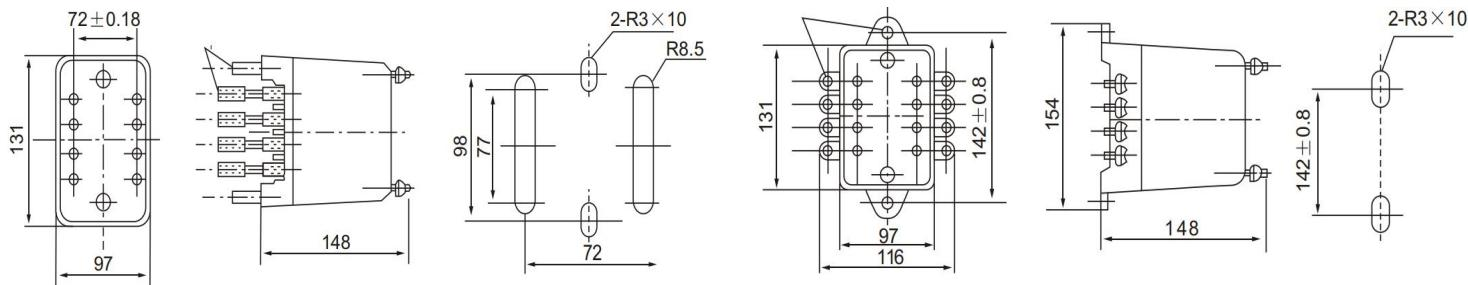
凸出式固定（后接线）Protruding fixing (rear connection)
